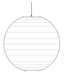
2. To secure the lantern open, insert the wire frame into the bottom of the lantern and pull the lantern up over the wire frame. Insert the top of the wire frame into the wire tabs on the top of the lantern, being careful to avoid tearing.
